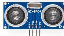
(Trigger), Echo (Receive) und GND (Ground).
